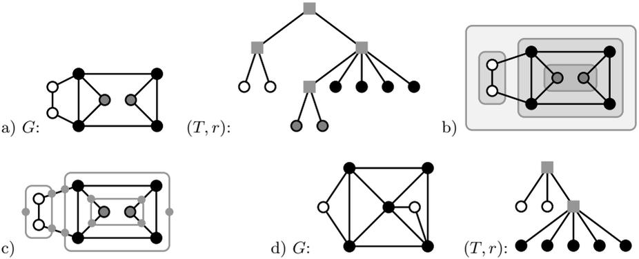
**Fig. 1.** a) A c-planar clustered graph that is not connected. b) A c-planar drawing of the clustered graph in a. c) The auxiliary graph associated with the c-planar drawing in b. Boundary cycles are grey. d) A connected clustered graph that is not c-planar. The correspondence of vertices of  $G$  and leaves of  $T$  is indicated by corresponding colors.
