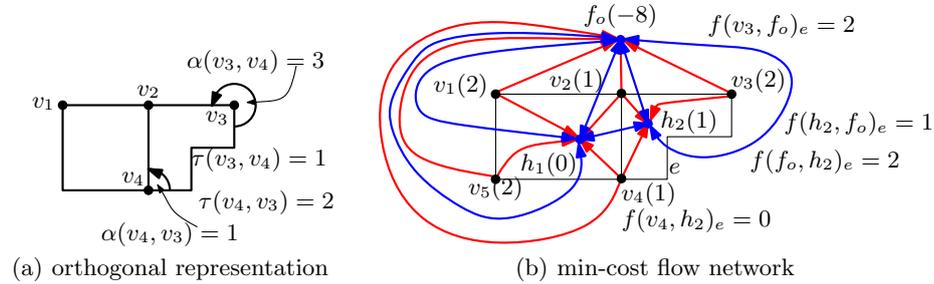
**Fig. 1.** Illustration of the approach of Tamassia [3] for solving the bend-minimization problem. In b) the directed arcs indicate the flow network. All arcs have infinite capacity, the bidirected blue arcs have cost one and the unidirected red arcs have costs zero. The node demands are indicated in brackets.
