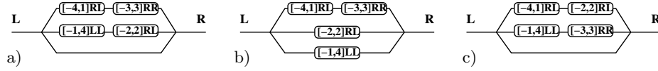
Fig. 1. a) A non-feasible platform assignment. b) A feasible platform assignment that is achieved with the first-fit algorithm. c) A feasible platform assignment that uses the minimum number of platforms.
