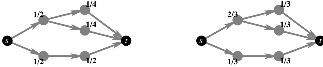
Fig. 2. Contribution of a single pair (s, t) to load ( left ) and betweenness ( right ).
